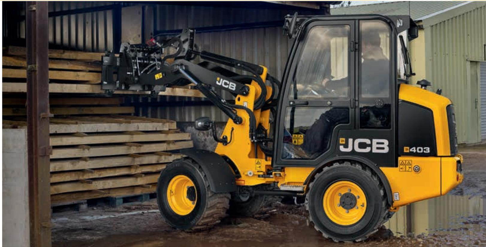
Compact wheel base and 45 degree steering articulation help to ensure tight turning circles and superb manoeuvrability.
