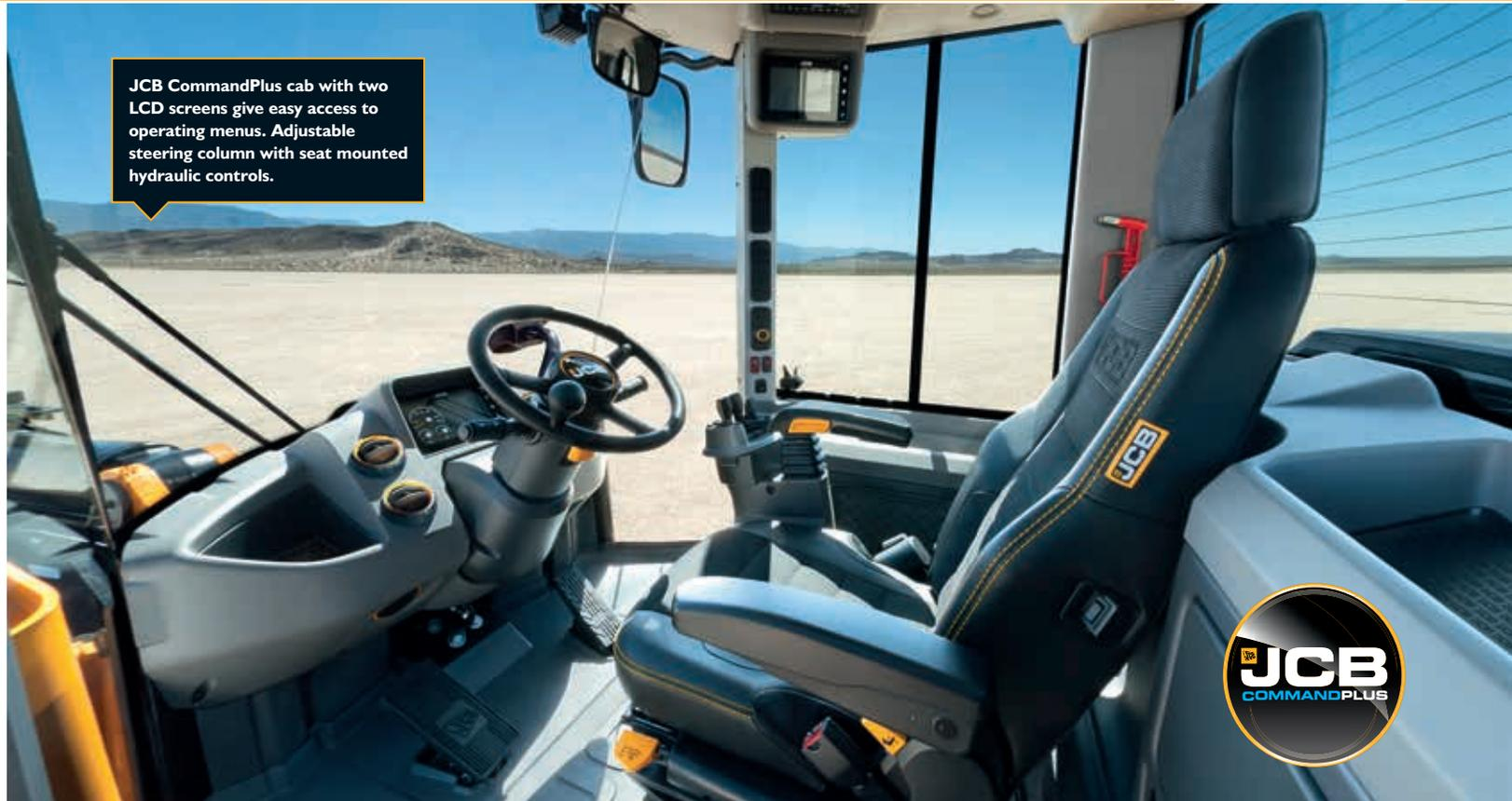
JCB CommandPlus cab with two LCD screens give easy access to operating menus. Adjustable steering column with seat mounted hydraulic controls.
