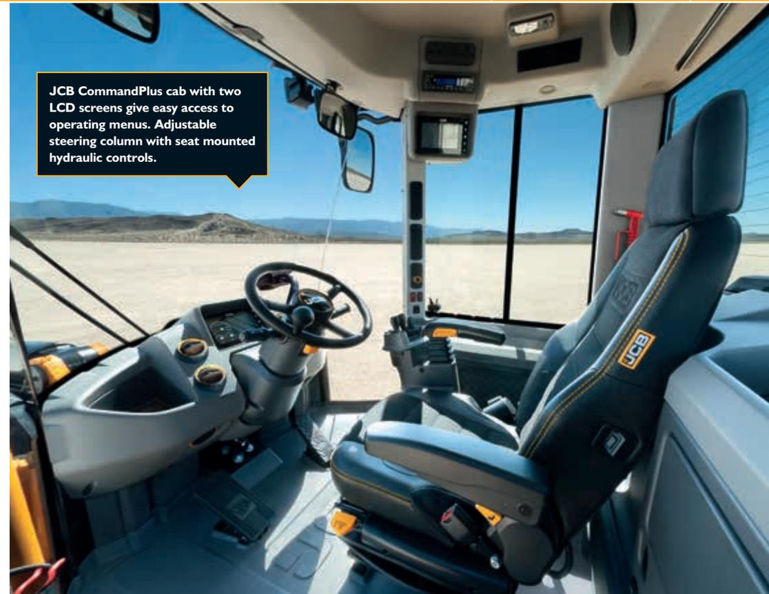
JCB CommandPlus cab with two LCD screens give easy access to operating menus. Adjustable steering column with seat mounted hydraulic controls.
